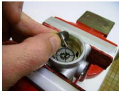
Next install the diaphragm. Bend between thumb and forefinger to make the installation easier. Push the diaphragm down to the inner shoulder and release.
