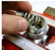
Using the bio adjusting spanner TL00008 unscrew the lock nut. (Turn anti-clockwise to unscrew)
