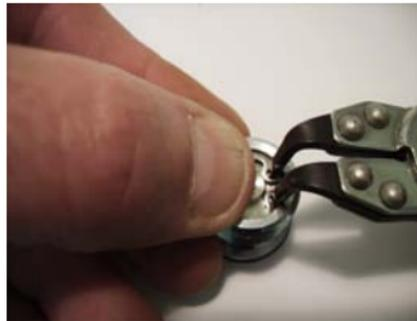
While compressing the retaining ring gradually reduce the downward pressure. The HP assembly should now disengage the module...
