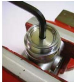
Do not replace the adjustable piston, outer diaphragm and outer diaphragm holder at this stage.
