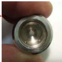
The pushrod assembly must be inspected for corrosion on the pin, also any bending of the pin. If any damage is noted replace the shaft.
