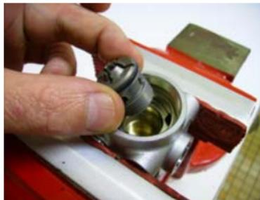
Using the 1<sup>st</sup> stage driver TL00002, screw the module into position. DO NOT tighten down hard. Tighten until the module bottoms and then back out approximately 1/64 of a turn. This will prevent the module locking into position after use.
