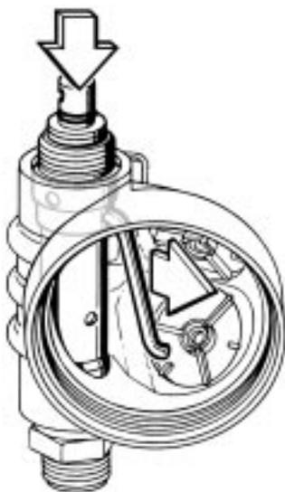
Fig. 21 - Retaining Sleeve Installation
