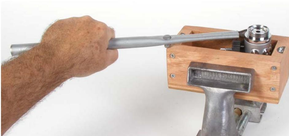
The box is sized and shaped, so that most brands of 1<sup>st</sup> stages can be dropped inside and positioned so that the cap, diaphragm clamp, yoke bolt, etc. can be placed just above the box's edge. As the technician applies force on the wrench being used, the regulator will
