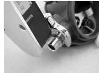
15. Install new o-rings (24&27) on either end of the M.P. hose. Thread the male fitting of the MP hose into the medium pressure port of the first stage and apply a torque wrench with a 9/16" crows foot to tighten to 40 (±2) in/lbs. Be certain that the first stage of the regulator is functioning properly and is delivering a medium pressure of 135 – 140 psi.
