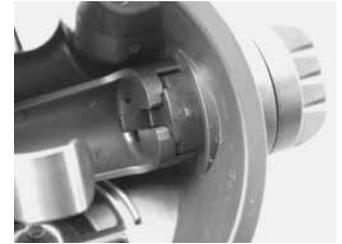
23. Install the exhaust valve cover (11) by positioning the two square holes in the cover over the mating two lugs on the box bottom (4). Swing it up into position and engage the latch. You should hear it "click" as it locks into place.
