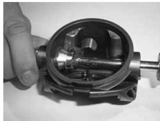
If the lever does not touch the tool, in other words, the lever is too low, screw the locknut back in until the lever reaches the correct height.
