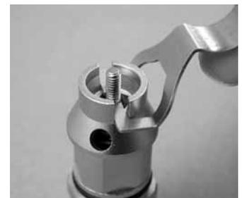
11. Place the washer (17) over the poppet shaft (22), followed by the locknut (16), with the flat side facing down. Being careful to avoid disturbing the lever (18), turn the locknut clockwise by hand to engage the threads of the poppet, and then apply a 1/4" nut driver to turn it further; only until 1 thread of the poppet shaft is visible above the top of the locknut.
