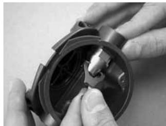
**WARNING:** The components that make up the valve subassembly are under spring tension. Disassemble according to instructions found in the next step. Failure to wear proper eye protection could result in an eye injury should the components (16-23) eject out of the valve body (19).
