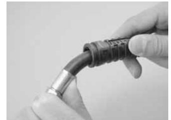
3. To remove the mouthpiece clamp (5), simply lift the lever on the cam latch with a screwdriver or thumbnail. Pull the mouthpiece (6) off. Inspect the mouthpiece to ensure it is free of any tears or cuts that may cause leakage of water into the second stage or other discomfort. Discard the mouthpiece or set it aside to be reused, depending on its condition.
