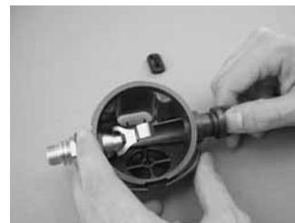
10. Remove and discard the O-ring (8) from the venturi switch (9), and closely examine the O-ring groove of the venturi switch to check for any nicks or scratches. Discard if found, or set it aside if it is in reusable condition.
