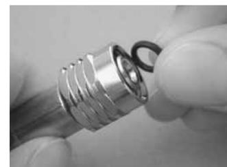
16. Attach the female fitting of the second stage medium pressure hose to the inlet fitting (13) of the second stage. Turn the swivel nut clockwise until finger snug.
