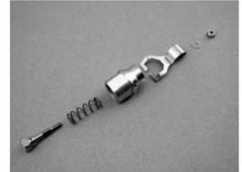
17. Closely inspect the shape and condition of the lever (18) to ensure it is not bent, corroded, or otherwise damaged. If any signs of damage or corrosion are found, discard the lever and do not reuse.
