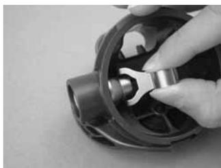
14. While holding the valve assembly (16-23) securely inside the box bottom (4) and the lever (18) depressed, mate the shorter threaded end of the inlet fitting (13) through the inlet port and into the valve assembly (16-23). Turn the inlet fitting clockwise by hand until finger snug, and then apply a torque wrench with a 3/4" (19mm) crow foot to tighten it to a torque measurement of 45 (±5) inch-pounds.
