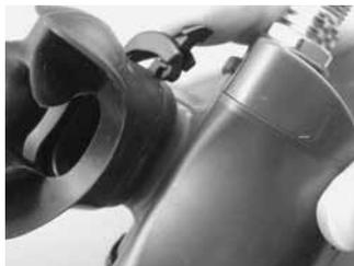
27. Attach the MP hose (25) to the second stage. Using an 11/16" (17mm) crow's foot, apply a torque of 40 (± 3) in. lbs.
