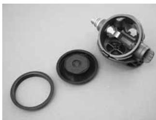
6. Once the front cover (1) has been removed, the release latch for the exhaust valve cover (11) becomes exposed. Using your finger, lift the release latch and swing the exhaust valve cover off of the lugs on the box bottom (4).
