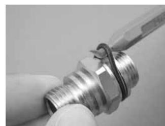
12. Apply a medium blade screwdriver to the slotted head of the crown (14) inside the inlet fitting (13), and hold the inlet fitting secure while turning the crown counter-clockwise to disengage the threads.
