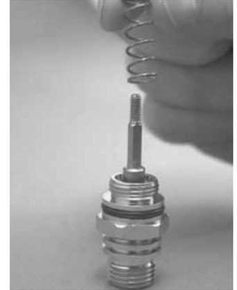
9. Hold the inlet fitting (13) secure, and mate the valve body (19) with poppet bearing down over the poppet shaft (22). Press the valve body downward to compress the spring while turning it clockwise to engage the threads of the inlet fitting, and then continue turning it slowly until the threaded portion of the poppet shaft stands outside the poppet bearing (20).
