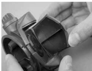
7. Inspect the exhaust valve and its seating surface underneath. The valve should be clean and supple. It should be free of any tears, holes or defects of any kind. It should have well defined edges. If it is dirty or compromised in any way, it must get replaced. The seated surface underneath the valve must be clean.
