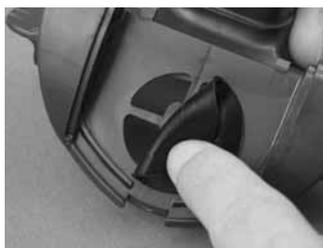
8. Using your finger, reach into the box bottom (4) and remove the retaining clip (7) for the venturi switch.
