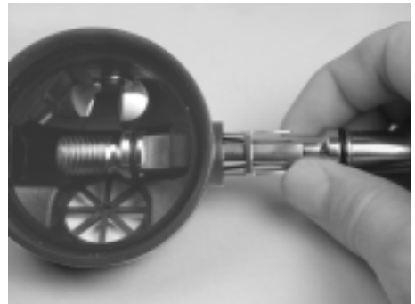
Figure 8. Depress the lever and slide the valve body out of the second stage
