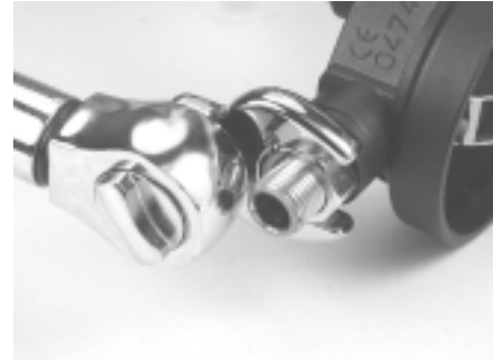
Figure 39. Install retaining nut and torque to 50 inch-pounds
