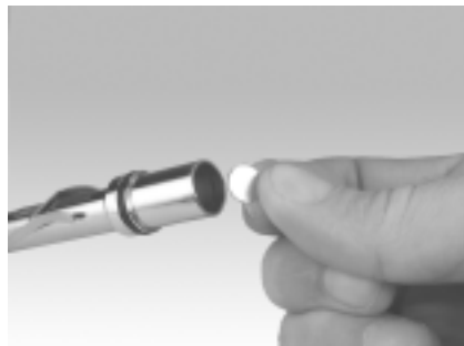
Figure 31. Install metal disk
