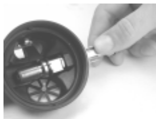
Figure 36. Depress lever and insert valve body
