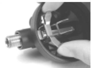
Figure 38. Install the retaining key over squared section
