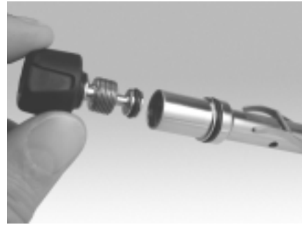
Figure 11. Unscrew adjustment knob to disengage threads, then pull straight out
