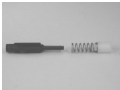
Figure 17. Separate poppet from balance chamber
