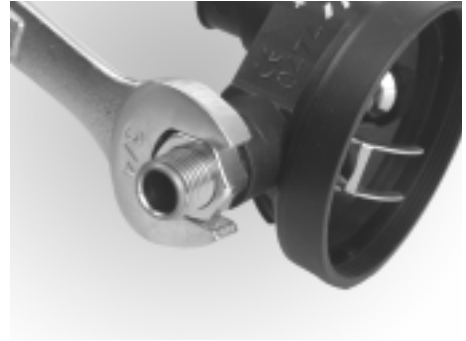
Figure 6. Remove retaining nut with 3/4-inch wrench
