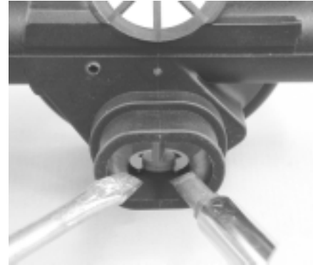
Figure 19. Push on both legs of the clip to remove
