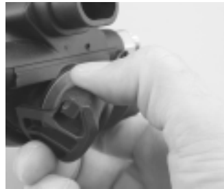
Figure 3. Press down on top corner of exhaust tee to remove
