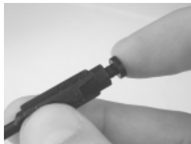
Figure 26. Install LP seat into poppet
