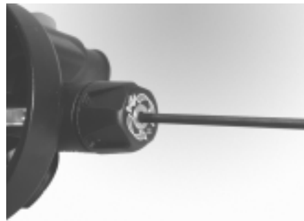
Figure 4. Remove retaining screw with 3mm hex wrench
