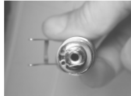
Figure 34. Inspect circlip to make sure it is properly seated
