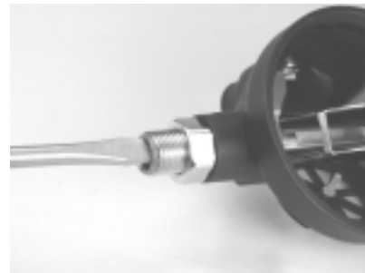
Figure 41. Tighten adjustable orifice until lever starts to drop
