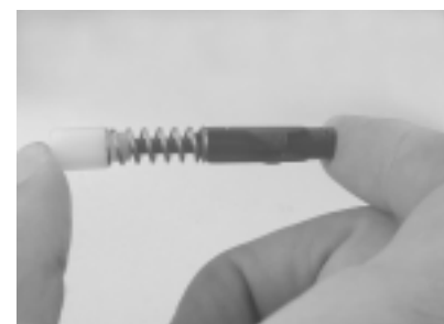
Figure 28. Install spring onto balance chamber; press poppet into balance chamber
