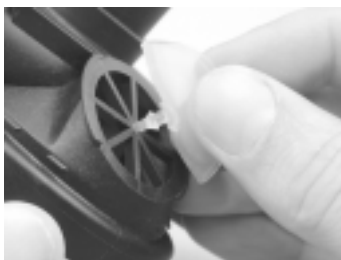
Figure 22. Install exhaust valve
