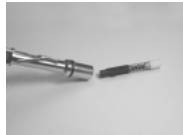
Figure 14. Poppet assembly removed from valve body
