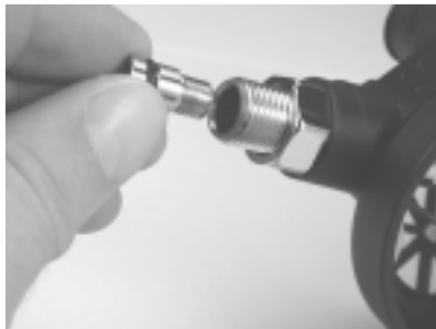
Figure 40. Install adjustable orifice into valve body
