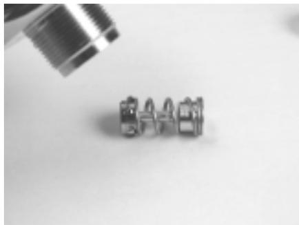
*Figure 11. Remove HP seat assembly*
