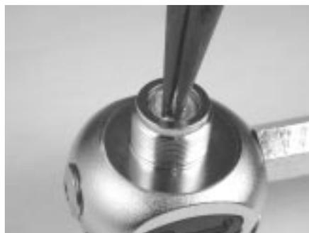
Figure 7. Remove filter retaining clip and filter
