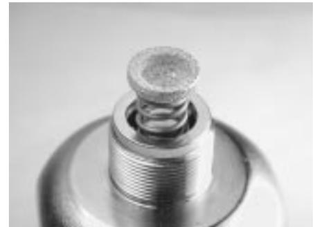
*Figure 23. Place filter, cup facing upward, onto spring*
