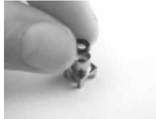
*Figure 20. Install O-ring*
