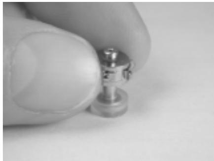
*Figure 14. Install sleeve onto HP seat*
