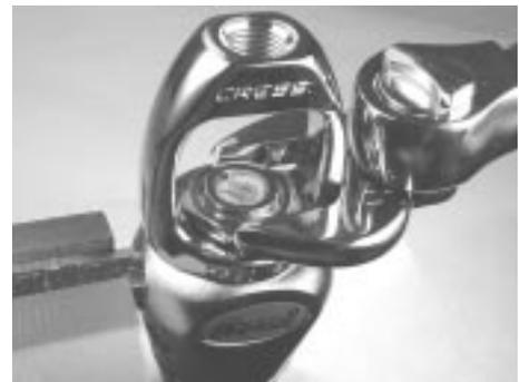
*Figure 35. Tighten retainer to 20 foot-pounds*
