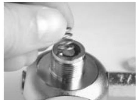
Figure 8. Remove balance chamber spring
