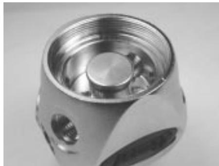
*Figure 27. Install pin support*
