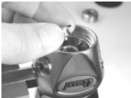
Figure 4. Remove the pin support
