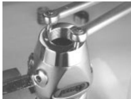
Figure 2. Remove spring retainer
