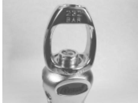
*Figure 33. Place yoke onto first stage body*
