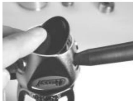
Figure 3. Remove diaphragm with a short blast of low pressure air
