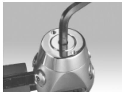
Figure 1. Mount first stage in vise and remove adjustment screw
