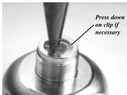
*Figure 24. Install filter retaining clip*
