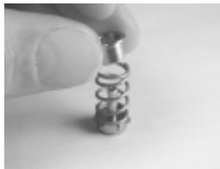
*Figure 17. Press balance chamber sleeve into spring*
