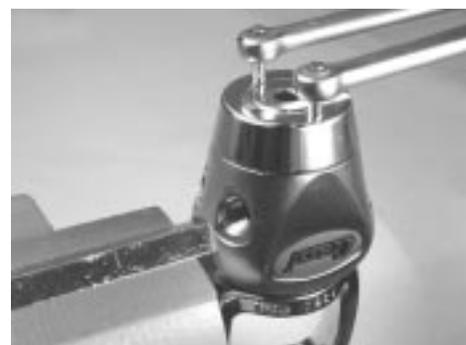
*Figure 36. Tighten spring retainer with adjustable face spanner wrench until it stops*
