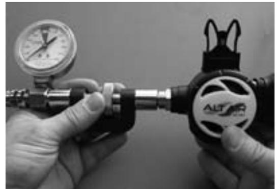
*Fig. 13 – Inline Adjustment Tool w/ IP Gauge*
