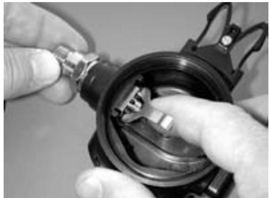
Fig. 11 – Installation of Inlet Fitting
