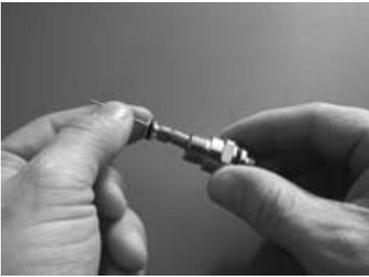
*Fig. 3 – Removal of Adjustable Orifice*
