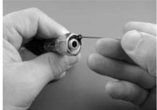
Fig. 2 – Removal of LP Hose O-ring
