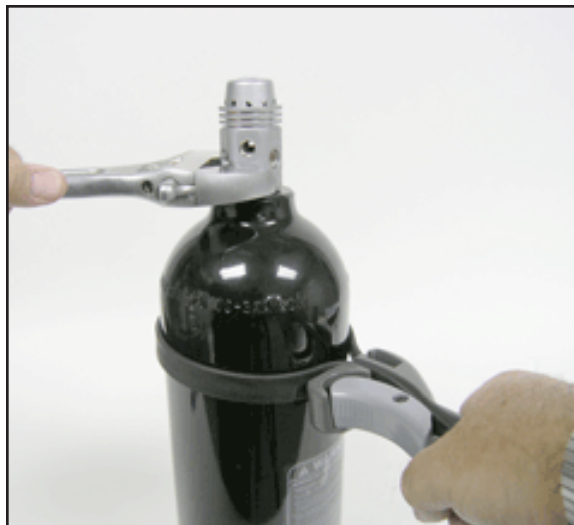
Removing the RaZor from the Cylinder
