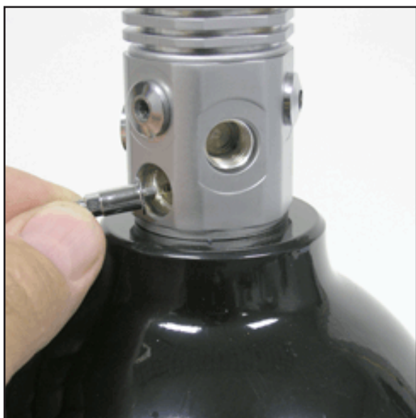
Plug Assembly (20) removal using Stem (25) as a tool.
