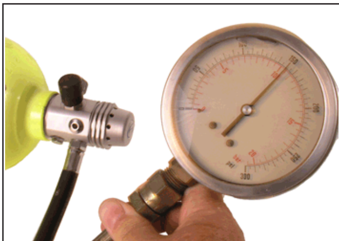
Checking the Intermediate Pressure with a Gauge
